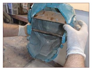
**FIGURE 2-43:** Keep moving the whole thing in order to keep goop from pooling in one place.
