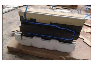
**FIGURE 1-70:** EL wire fitted into the grooves on the side of the forward section
