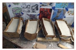
FIGURE 9-15: The molds filled with plaster
