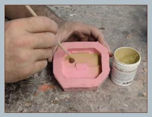
FIGURE 6-17: Dusting the mold with powdered brass
