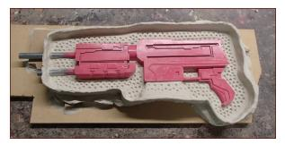
**FIGURE 7-27:** The clay bed, complete with a raised drip wall around the outside
