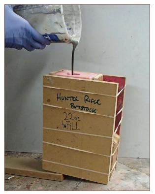
FIGURE 7-16: Pouring in some resin
