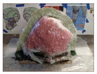
FIGURE 8-19: Fiberglass patches laid into the wet resin
