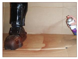
**FIGURE 13-27:** Holding the spray can too far away from the surface will cause paint droplets to form in the spray pattern.
