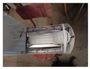
FIGURE 10-15: The back shell of the space heater removed
