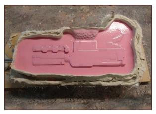
FIGURE 7-42: The print coat poured on the second half of the prototype
