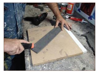
FIGURE 3-2: Making a straight cut in foam
