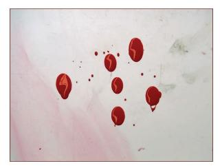
FIGURE 13-56: Oblong drops created by dripping paint onto an inclined surface
