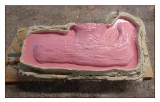
FIGURE 7-43: The thickened rubber jacket
