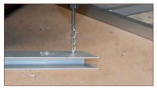
FIGURE 10-5: Drilling the frame
