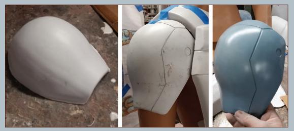
**FIGURE 9-40:** Hunter's shoulder formed as a single layer of plastic (left), two layers with details cut into the outer layer (middle), and glued together with paint and weathering (right)
