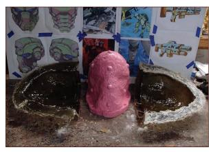
FIGURE 8-31: The mother mold removed from the rubber jacket
