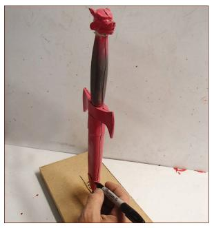
**FIGURE 6-23:** Marking the sides of the prototype and the bottom of the mold box where the mold will be cut
