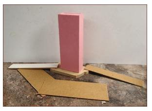
FIGURE 6-29: Careful disassembly of the mold box
