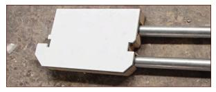
**FIGURE 1-69:** The conduit held in place once the piece is skinned over with the first layers of plastic
