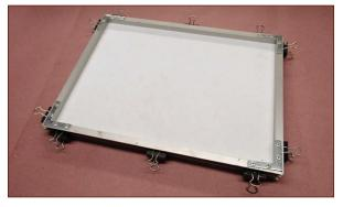
FIGURE 10-36: The plastic sheet in the clamping frame
