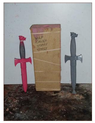
FIGURE 6-38: The prototype, the mold, and the first cast part
