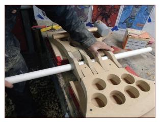
**FIGURE 1-23:** Keeping the handle in place makes sure that the holes will line up properly.
