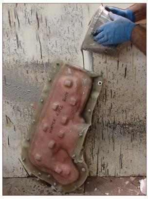
FIGURE 7-60: Pouring a casting
