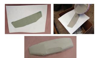
**FIGURE 9-4:** Pulling a plaster copy of the forming buck from a formed sheet
