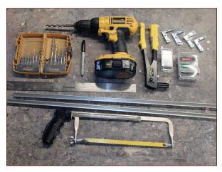
**FIGURE 10-1:** A drill with a  $\frac{1}{8}$ " bit, a ruler, a permanent marker, a pop rivet gun, 90° corner brackets, pop rivets, washers,  $\frac{1}{2}$ " aluminum C-channel stock, and a hacksaw
