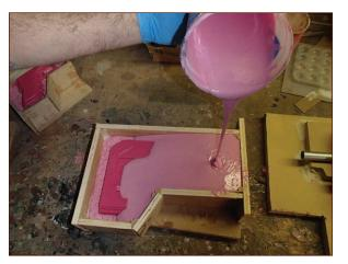
FIGURE 7-11: Pouring the second half just like the first half
