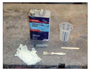
FIGURE 2-35: Tools for coating with fiberglass resin
