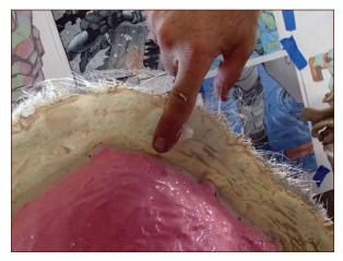
**FIGURE 8-25:** Goobering the petroleum jelly onto the flange with a fingertip
