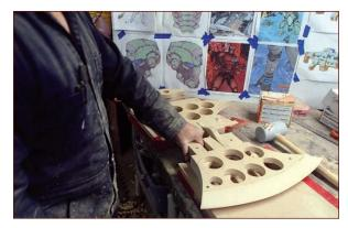
**FIGURE 1-22:** The blades propped up on some scraps of MDF so they'll stay straight
