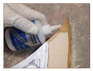
**FIGURE 1-41:** Soaking the edges of the blade with cyanoacrylate glue for strength
