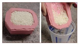
FIGURE 6-12: Using rice to determine casting resin volume
