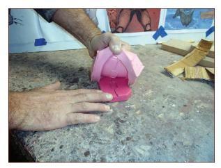
FIGURE 6-10: Peeling the mold off the prototype
