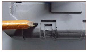
**FIGURE 7-63:** Tiny bubbles are the bane of a prop maker's existence, and they must be destroyed.
