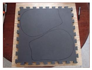
FIGURE 3-26: The parts traced onto the foam, then cut out with a knife before sanding the edges smooth
