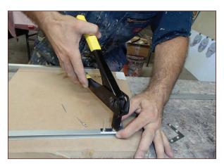
FIGURE 10-6: Riveting
