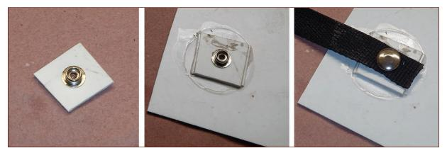
FIGURE 14-4: A good method of attaching snaps to vacformed armor without a visible attachment on the surface
