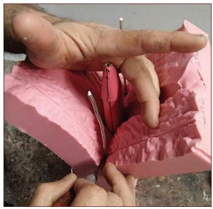
**FIGURE 6-33:** Cutting both sides will make it easier to pry the mold open.
