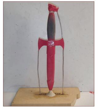
FIGURE 6-25: Vents added to allow bubbles to flow out of the mold
