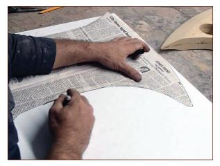
FIGURE 1-31: The shape traced onto the plastic sheet
