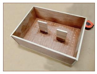
FIGURE 9-24: The grid drilled
