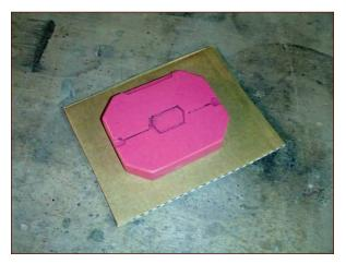
FIGURE 6-3: Prototype securely anchored to a piece of cardboard
