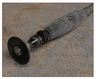
FIGURE 8-34: The cut-off wheel
