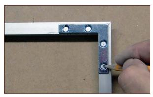
FIGURE 10-4: Marking the locations to drill
