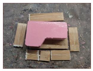
FIGURE 7-12: The disassembled mold box
