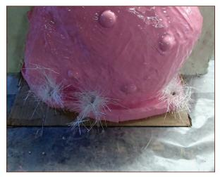
FIGURE 8-17: Peg holes loosely stuffed with fiberglass
