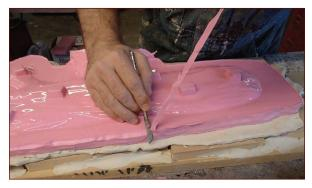
FIGURE 7-35: Cleaning up the edge of the rubber
