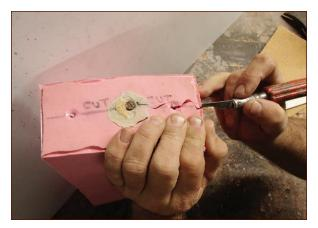
FIGURE 6-31: An initial scrpentine cut in the top of the mold
