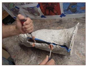
**FIGURE 9-13:** Using a pair of screwdrivers to gently pry apart the two halves of the plaster mold
