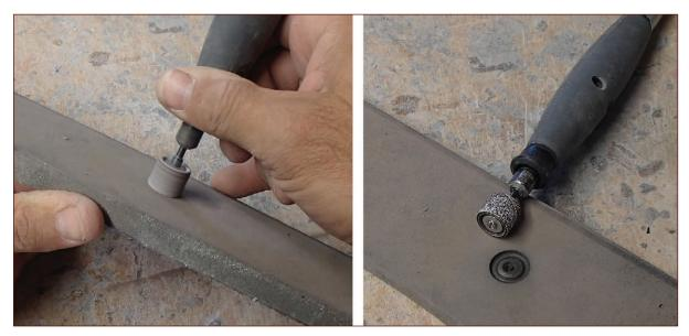
FIGURE 3-57: Simulating a rivet head with the tip of a sanding drum on a rotary tool
