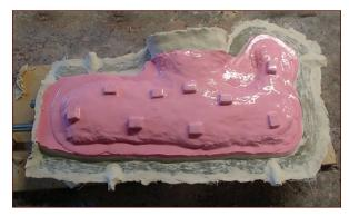
FIGURE 7-48: Lumps of clay along the edges of the mother mold
