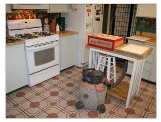
**FIGURE 9-29:** The forming platen plugged into the shop vacuum and positioned conveniently near the oven
