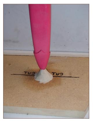
FIGURE 6-24: A sprue made out of clay
