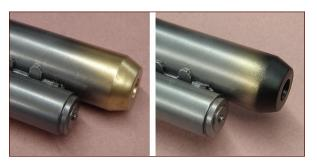
**FIGURE 13-53:** A bit of gold (left), mostly covered with black (right), makes for an even more believable bit of heat-treated metal.
