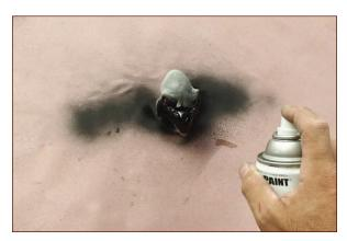
**FIGURE 11-8:** Start spraying before the can is aiming at the object and continue after sweeping past.
