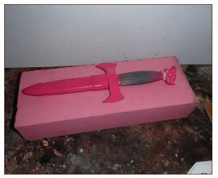
FIGURE 6-35: The prototype removed from the cut mold.
