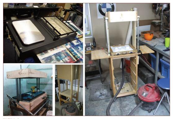
FIGURE 10-12: Just a few examples of homemade vacforming machines
