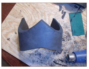
FIGURE 3-49: The curved rib piece
