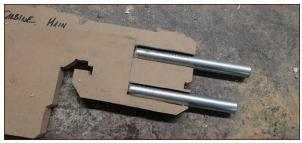
FIGURE 1-53: Notch with a piece of  ${\mathscr V}''$  metal electrical conduit fitted into it.
