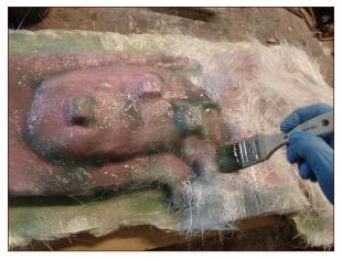
FIGURE 7-38: Brushing resin into (and bubbles out of) the fiberglass mat
