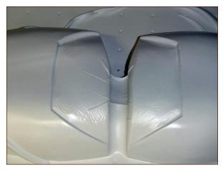
FIGURE 9-34: Webbing caused by having two forming bucks too close together
