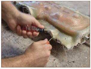
FIGURE 7-56: Prying the two halves of the mother mold apart
