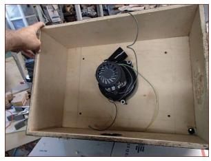
FIGURE 10-27: The vacuum motor installed in the bottom of the platen
