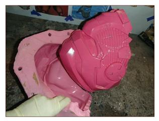
FIGURE 8-33: Removing the prototype from the rubber jacket
