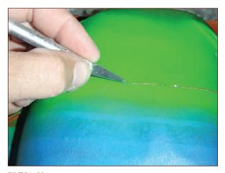
**FIGURE 11-24:** Once you've cut the bond along the edge of the tape, remove it as you normally would before you remove the tape.
