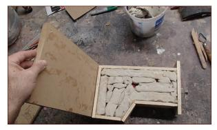
FIGURE 7-9: The mold box flipped over with its bottom removed
