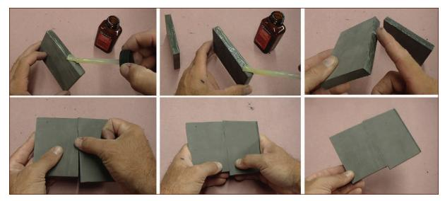
FIGURE 3-6: Joining two pieces with contact cement
