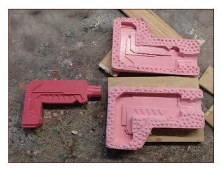
FIGURE 7-13: The demolded prototype
