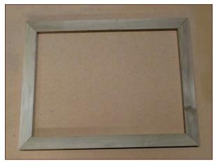
FIGURE 9-19: Wooden parts for one side of the vacforming frame
