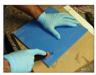
FIGURE 3-3: Cutting a curve
