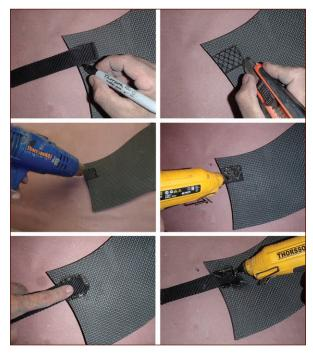
FIGURE 14-12: Gluing straps to EVA foam
