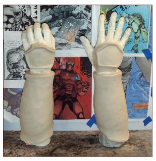
**FIGURE 9-6:** There's no easy way to get this forearm armor formed in one piece without the plastic sheet locking onto the forming buck.
