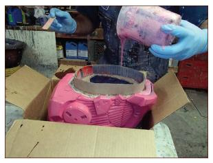
FIGURE 8-5: Filling the undercuts with silicone while the prototype is upside-down
