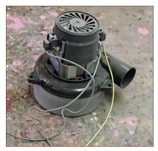
FIGURE 10-25: The driving force behind the vacuum cleaner
