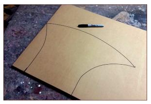
FIGURE 1-15: The shape of half the blade drawn out on the sheet
