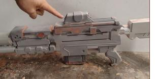
**FIGURE 1-84:** The sight fitted into place over the battery pack cutout on top of the rifle
