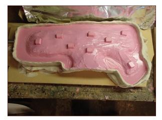
FIGURE 7-31: Registration keys added to the surface of the mold
