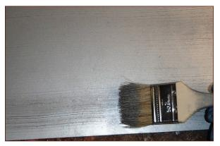
**FIGURE 12-4:** Adding brush marks to the smooth coat of sprayed silver paint
