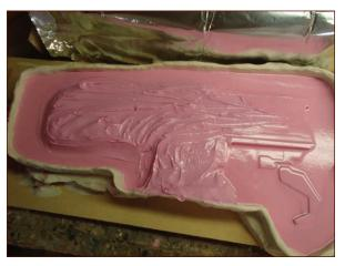
**FIGURE 7-30:** The rubber jacket halfway frosted with thickened silicone
