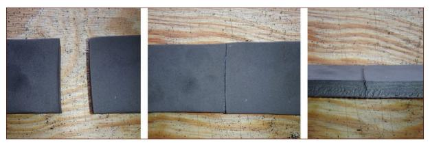
FIGURE 3-7: Butt joint. Stop giggling.
