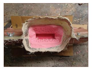
FIGURE 7-53: The magazine well prepped for molding
