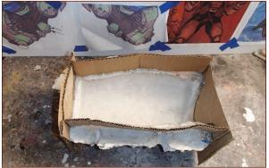
**FIGURE 9-14:** The open end of the molds closed up with corrugated cardboard and hot glue
