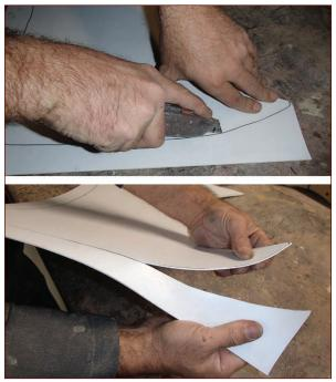
FIGURE 1-32: Score and snap—the quick and easy way to get shapes out of styrene
