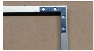
FIGURE 10-3: A corner fitted with an angle bracket
