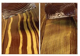
**FIGURE 12-22:** The straight edges of the graining tool are also textured to simulate other wood grains.
