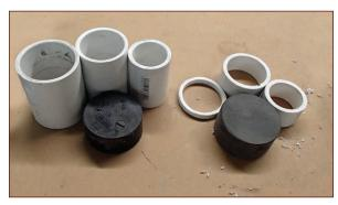
**FIGURE 1-44:** Boring pipe fittings (left) stop being recognizable (right) with just a bit of love from a miter saw and a sanding block.
