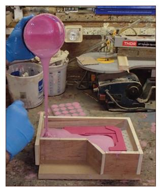
FIGURE 7-8: Pouring rubber with style
