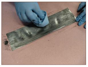
**FIGURE 12-6:** Gently removing most, but not all, of the black paint with a rag leaves streaks behind.
