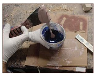
**FIGURE 2-40:** Blob of Bondo blobbed into mixing cup of resin to make a superblob
