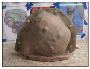
FIGURE 8-36: The reassembled mold; ready to roll
