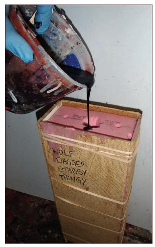
FIGURE 6-37: Pouring slowly and carefully in order to avoid bubbles
