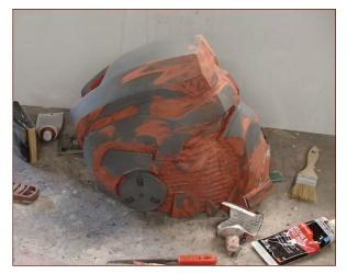
FIGURE 2-54: A few tiny holes filled with spot putty
