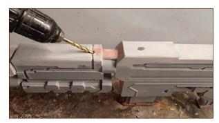
FIGURE 1-87: Holes drilled to feed EL wire through
