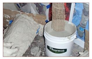
**FIGURE 9-11:** Plaster-soaked strips of burlap laid into the stillwet plaster will make for a stronger mold.
