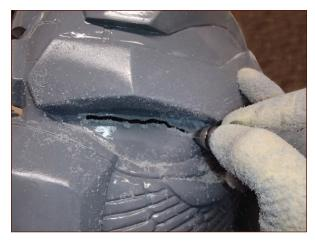
**FIGURE 8-44:** Rough trimming the eye holes, leaving material around the edges to be cleaned up later
