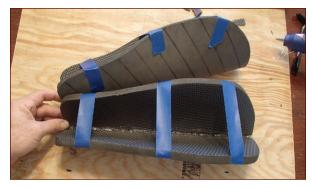
**FIGURE 3-27:** Masking tape holds the pieces in position while you're waiting for the glue to cure and the foam to cool.
