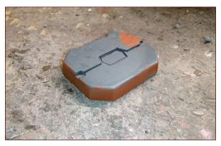
FIGURE 1-12: The edges coated with a smidgeon of spot putty
