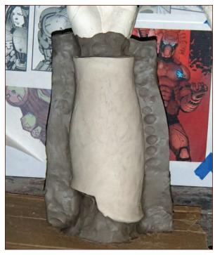
FIGURE 9-7: A parting wall made of water-based clay
