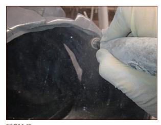
FIGURE 8-45: 80-grit sanding drum—because sometimes roughness is the best path to smoothness
