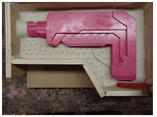
**FIGURE 7-7:** The finished clay bed, complete with dimples to form registration keys
