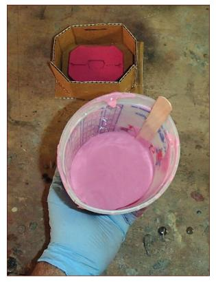
FIGURE 6-5: Properly mixed silicone is all one uniform color.
