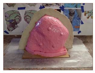
FIGURE 8-16: The clay parting wall
