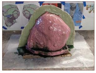
FIGURE 8-18: The mold coated with resin
