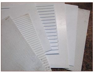
**FIGURE 1-9:** Textured styrene sheet intended to look like miniature siding, diamond plate, and roofing materials for tiny buildings.
