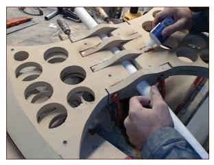
FIGURE 1-25: Applying glue to the seams
