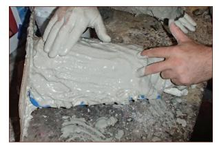
FIGURE 9-9: Thickening the mold with more plaster
