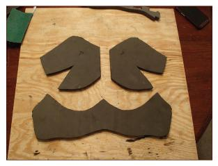
FIGURE 3-48: Cutting out the foam parts based on the paper templates
