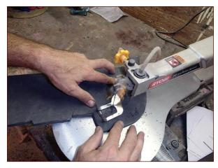
FIGURE 3-5: The scroll saw makes quick work of cutting foam.
