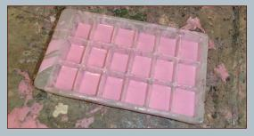
**FIGURE 7-29:** The half-filled ice cube tray makes good registration keys.
