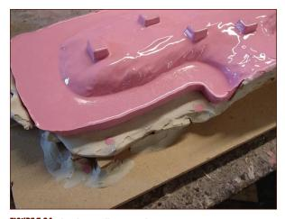
FIGURE 7-34: The drip wall removed
