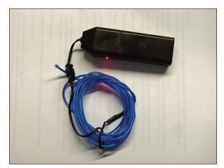
FIGURE 1-65: A neat little prepackaged EL wire system
