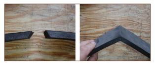
**FIGURE 3-8:** Viewed from end on, the angle-cut (or *mitered*) pieces join together to create a corner.
